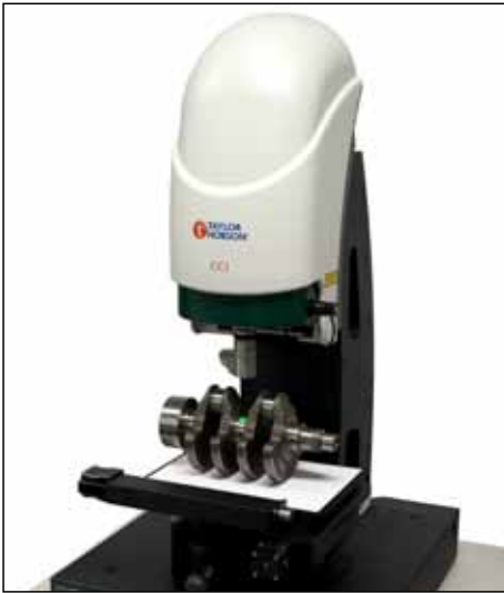
The CCI MP-HS XL is optimized for the measurement of large components without compromising the resolution
