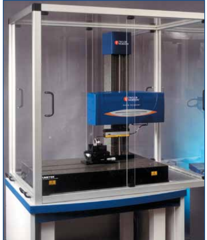
Form Talysurf PGI 1200 with environmental cabinet
