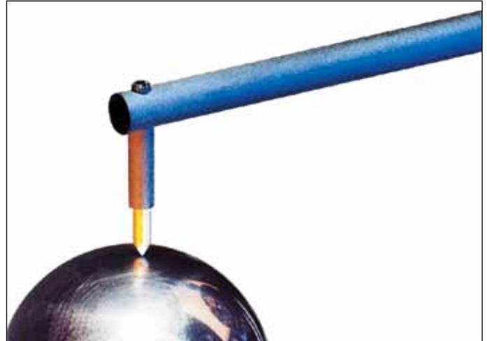
contacting stylus inspection methods are preferred for measuring high precision bearings
