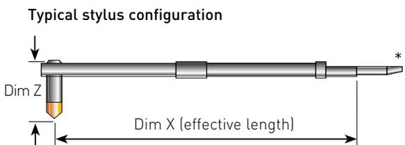
\* Improved spigot design provides easy interchangeability along with rigid mounting for overall stiffness and measurement repeatability
