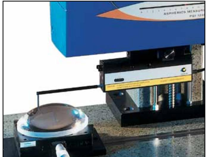
calibration over a spherical artifact checks gauge linearity, stylus condition and processor functions
