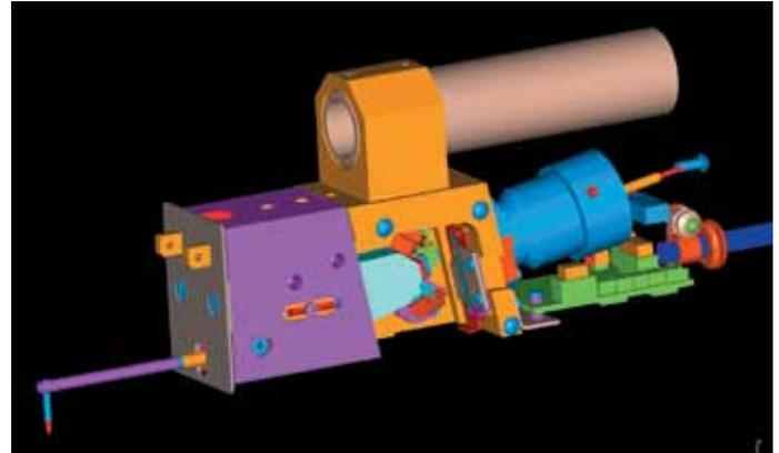
CAD rendering of PGI gauge mechanism
