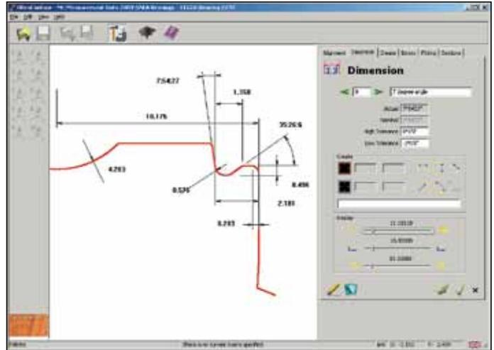
contour analysis software (detail of bearing seal profile)
