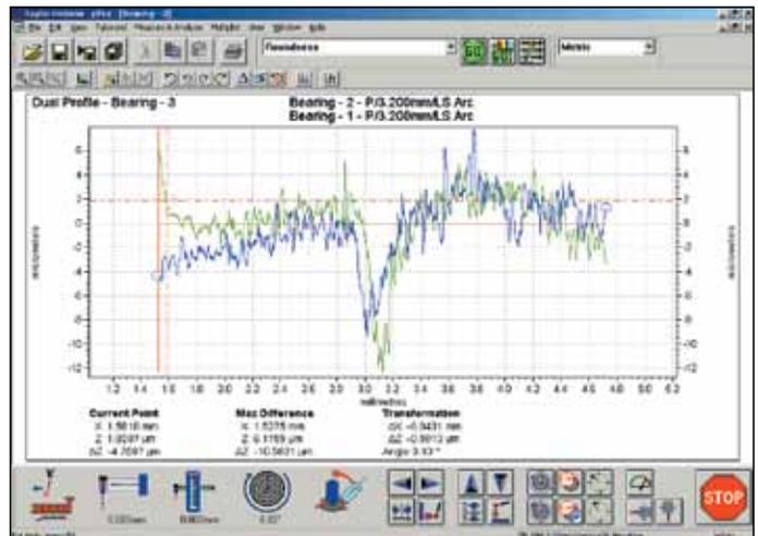
dual profile software (detail of track profile at two locations)
