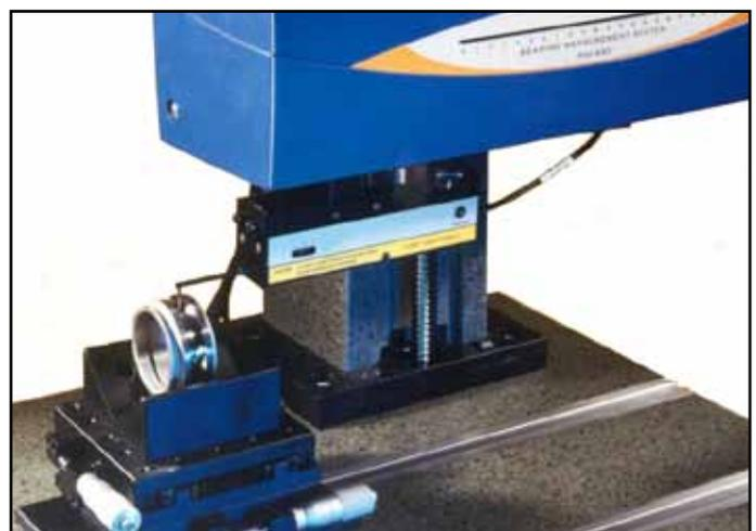
measurable form features may be aspherical, spherical, concave, convex, internal or external
