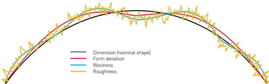
The elements of a surface are inseparable in the function of a component (not drawn to scale)
