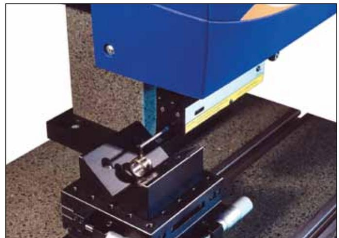
Form Talysurf PGI 420 with 4mm gauging range is ideal for small and miniature bearings
