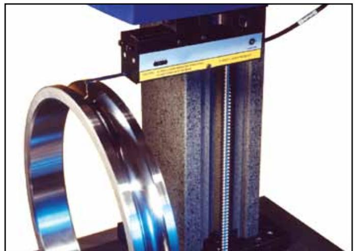
measure dimension, form and texture at once with a single traverse over curved surfaces
