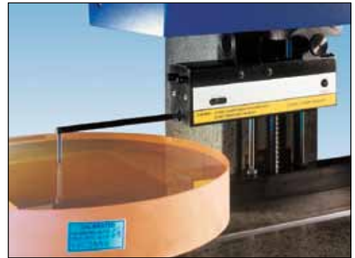
an optical flat is used to calibrate horizontal straightness of the 200mm traverse unit which serves as an absolute reference datum
