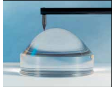
vertical gauge range is 12.5mm (expandable to 25 or 38mm) to handle optical components with large SAG or slope dimensions
