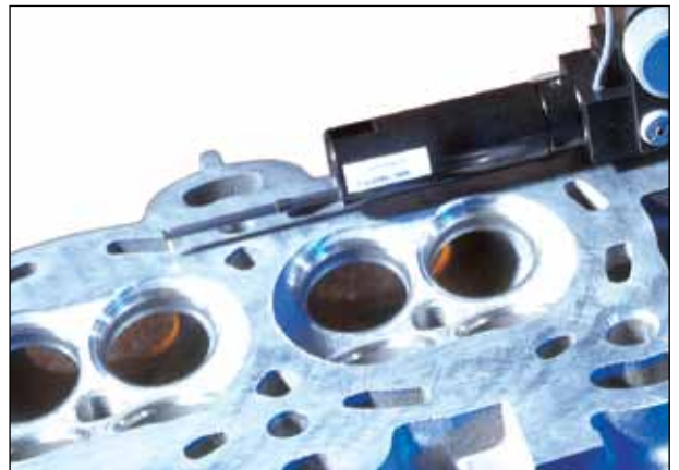
High resolution skidless pick-up is necessary for straightness and waviness measurements
