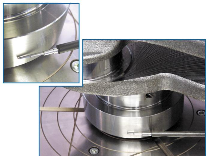
Twist measurement on a crankshaft using a Talyrond with a diamond tipped stylus arm mounted in the Talymin 5 gauge
